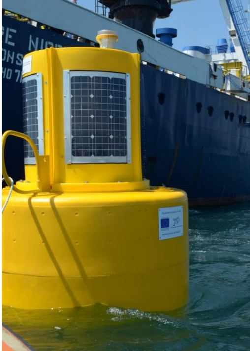
EUXINUS network – Automatic marine gauge
