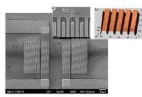
GaN based 5.3 GHz SAW structure (A. Muller; G. Konstantinidis et al. *IEEE Electron Devices Lett.*, vol 31, no. 12, 2010, pp 1398-1400)
