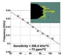
The temperature dependence of the resonance frequency of SAW single resonator having 50µm length fingers from  $S_{11}$  on wafer parameter measurements
