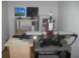
The millimetre wave characterization equipment up to 110 GHz
