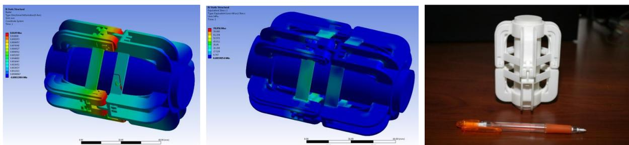
ANSYS simulation of the torque sensor behaviour under the action of centrifugal force at 10.000 rpm. Left: radial displacement; Middle: von Mises stress; Right: Beta version of the torque sensor
