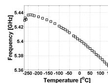
The temperature dependence of the resonance frequency obtained for SAW diced chips from run 3 mounted on ceramic substrate obtained from  $S_{11}$  measurements in the range -250° - +150° C
