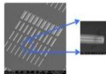
Platinum deposition was used for fixing the CNTs across V-shaped trenches in order to measure their mechanical properties
