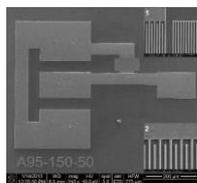
Single resonator SAW test structure; the two insets present details of the IDTs and reflectors (fingers and interdigit spacing 200 nm) manufactured at IMT using advanced nano-lithographic processes (Run 3)
