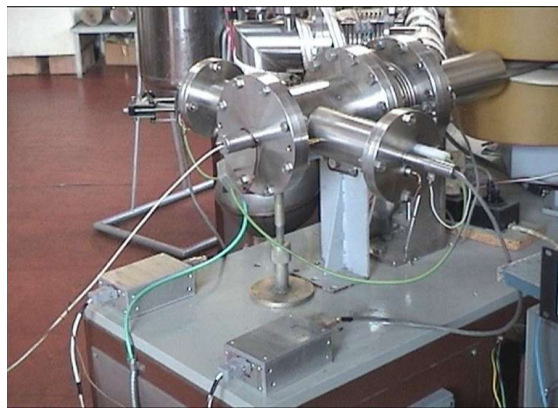
Figure 5. The double collector system inserted in the structure of the SMIT-1 spectrometer.
