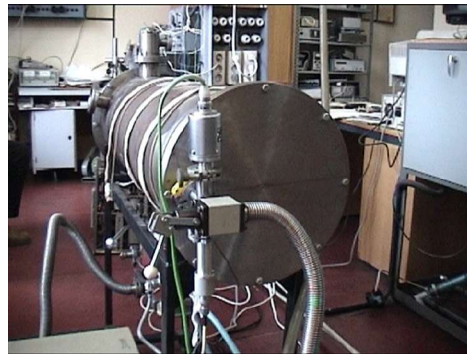
Fig 5. General view of the flight tube and vacuum system
