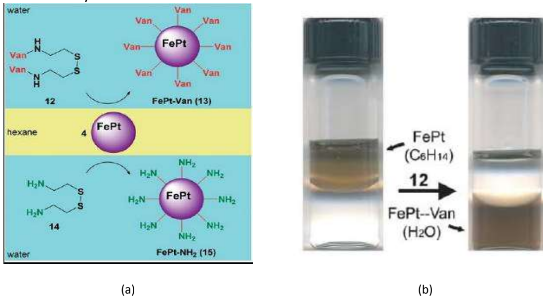
(a) Vancomycin attaching reaction to FePt nanoparticles (b) FePt in hexane and a FePt-vancomycin in water [1].
