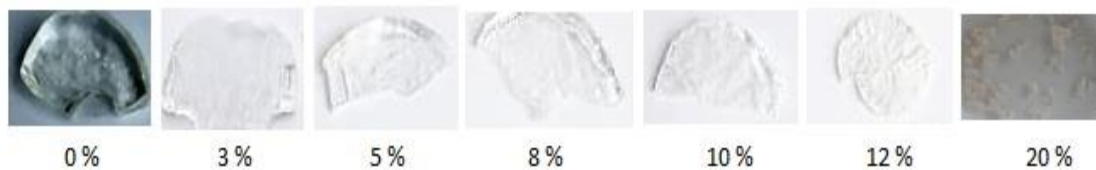
x\text{Tb}_4\text{O}_7 \cdot (100-x)[4\text{B}_2\text{O}_3 \cdot \text{PbO}] , where x=0-20 mol % \text{Tb}_4\text{O}_7
