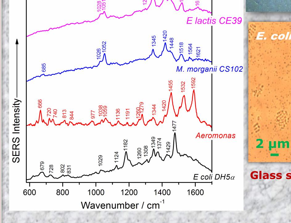
SERS spectra of the tested Gram-positive and Gramnegative bacteria on Polysine<sup>™</sup> Microscope Adhesion Slides using 532 nm laser line (A). SERS spectra of the *E. coli* strains on Polysine™ Microscope Adhesion Slides, obtained using 532 nm laser line (B).
