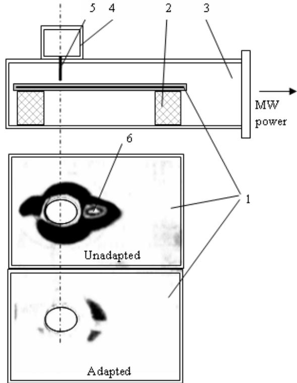
**FIGURE 6.** Coaxial to waveguide adapting measurements with patented termographic transducer: 1-termographic transducer sheet showing the MW power distribution for adapted and unadapted cases; 2-dielectric support (honeycomb material); 3-microwaves waveguide; 4- CW magnetron; 5-magnetron antenna; 6-trace of the microwave power leakage in the unadapted case.
