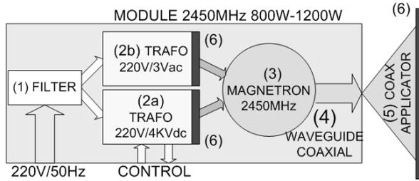
**FIGURE 2.** Microwave generator structure: 1-low pass filter (LPF), 2a-anode supply, 2b-filament supply, 3-magnetron, 4-waveguide to coaxial, 5-coaxial applicator, 6-isolation barrier.
