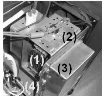
**FIGURE 7.** MW generator appearance: (1) CW magnetron, (2) temperature switch, (3) waveguide, (4) power supply
