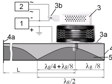
**FIGURE 4.** Magnetron placement on the waveguide: 1-anode power supply, 2-filament transformer, 3-magnetron, 3a-anode, 3b-filament and cathode, 4-waveguide, 4a-waveguide flange, 5-electric field distribution.
