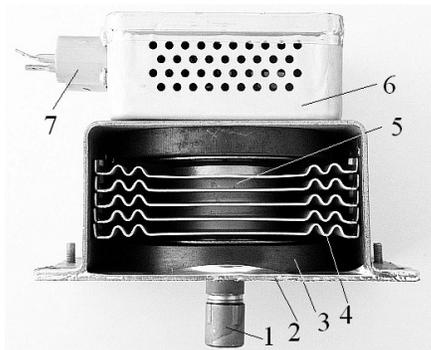
**FIGURE 1.** The CW magnetron aspect: 1-antenna, 2-mounting plate, 3-magnet, 4-heat sink, 5-anode, 6-filter box, 7-cathode and filament terminals.
