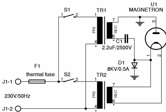
**FIGURE 3.** Classic magnetron power supply: TR1-anode transformer, TR2-filament transformer, F1-thermal fuse, C1 and D1-voltage doubler, S1 and S2-zero cross electronic switch, U1-CW magnetron.
